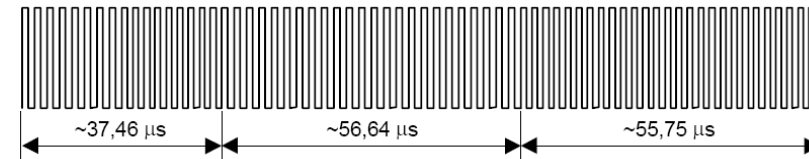
logic 0, ~ 424 kHz, 484 kHz (27 periods)
