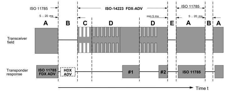
**Cycle A:** The transceiver reads the ISO 11785 frame. With the bits defined in the reserved field the transceiver detects, that an advanced FDX-ADV transponder is in the interrogation field. **Cycle B:** The transceiver switches off the interrogation field for at least 5 ms in order to reset the
